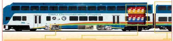
The DMU contains propulsion engines and passenger seating in one railcar, unlike a locomotive hauling coaches
