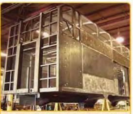
The double deck DMU structure also meets the FRA's newest 49 CFR Part 238 structural requirements.
