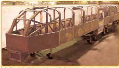
On February 26, 2002, the single level DMU was tested and shown to be the only self-propelled commuter railcar to meet the FRA's newest 49 CFR Part 238 structural requirement.
